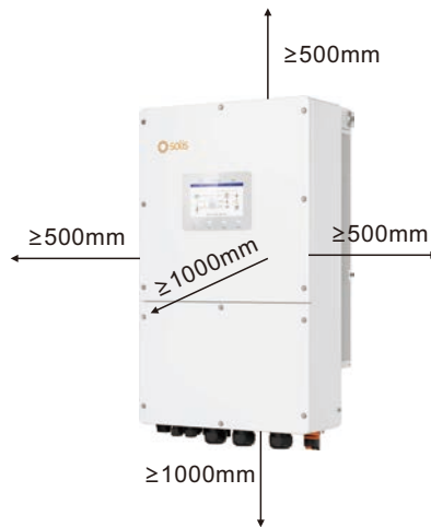
Figure 3.5 Inverter Mounting Clearances
